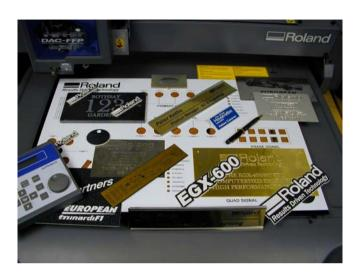
The EGX-600 is an extremely versatile engraving machine. It can engrave all types of plastic, aluminium, brass, glass, wood and even stainless steel. But, before you engrave, you have to decide what cutter to use and how to set up the machine. Following are quick reference notes on the different ways to engrave.
